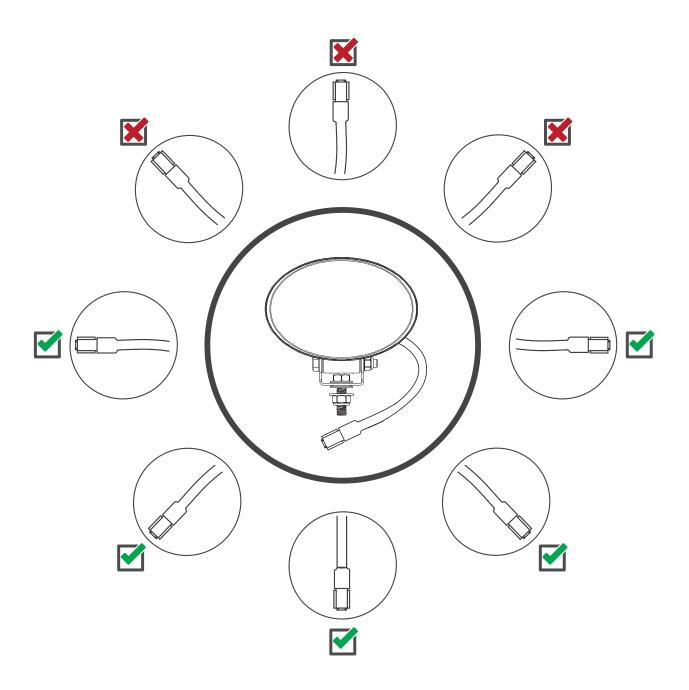
Do not point the connector plug upwards in any ways or water can get in. Point it down or horizontally.
