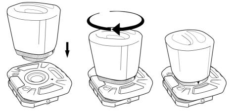
Step 1. Target the Triangle mark on the shield with the one on the lamp.
