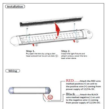
Lens: Polycarbonate, Clear diamond Base: Aluminum anodized in Silver Size: 383.1 (L) x 70.4 (W) x 18 mm (H)
