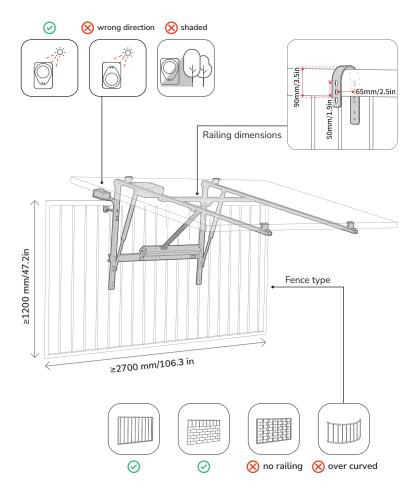
Please install the product in a position where it will not easily be shaded, so as not to affect the tracking performance of the rain-light sensor.
