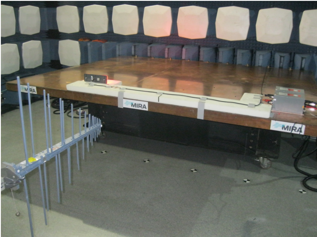
Plate 3 Annex VII and VIII, Radiated Emissions, Log Periodic IMG_1400
