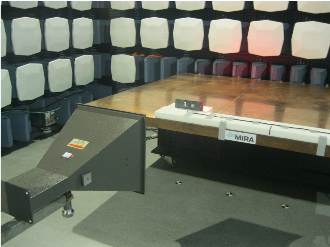
Plate 5 Annex IX, Radiated Immunity, Horn Antenna IMG_1409
