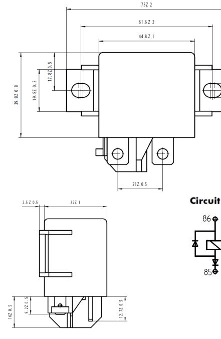
Nominal Coil Voltage: 12V Rated Current (Coil): 150mA Power Consumption: 1.8W Coil Resistance: 80Ohm +/-10% Contact Type: Normally Open Contact Material: Tungsten Nominal Current: 75A Operation Life Electrical: 100.000 Operation Life Mechanical: 1.000.000 Features: 2x Diode Temperature Range: -40 to +85°C Pulling Time: <10 s Drop Out Time: <10s Weight: 95g Insulation Resistance: 100 M Ohm
